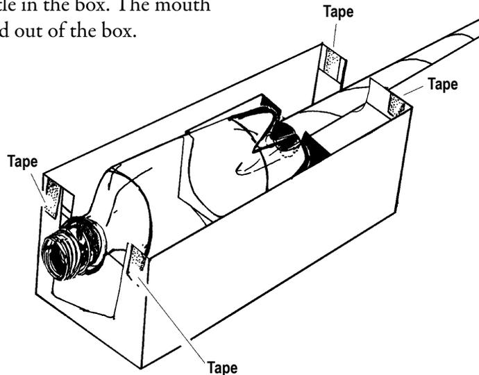
3. Using the cool-melt glue gun, run a small bead of glue along one end of the air tube. Press the glued edge of the air tube to the sanded bottom of the plastic bottle. Make sure the holding fixture and tube are aligned and that the tube is straight. Let the glue set for a few minutes.
