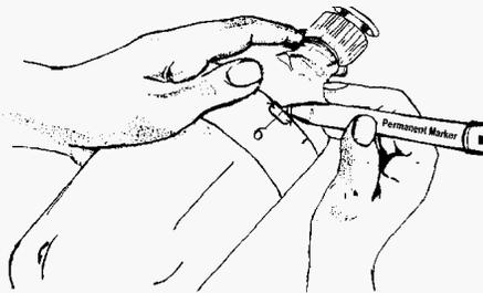
tical lines for fin placements, align each of the marks on the bottle against a door frame. Using the permanent marker, draw a 1-3/4" line straight down from the mark.
