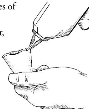
marks on the rocket body. Make sure the fin is perfectly aligned with the mark. Let the Stratoblaster set until the glue is dry. Repeat this step for the other two fins, and allow the glue to dry before moving to the next fin.
