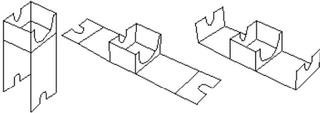
2. Using scissors, cut through the ends of the box to expose the U shaped holding fixture guides. Tape the holding fixture to the box with transparent tape. Place the plastic bottle in the box. The mouth of the bottle should extend out of the box.
