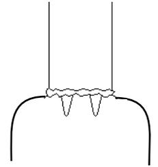
5. Return the bottle and tube assembly to the holding fixture to dry. Make sure the bottle and air tube stay aligned.
