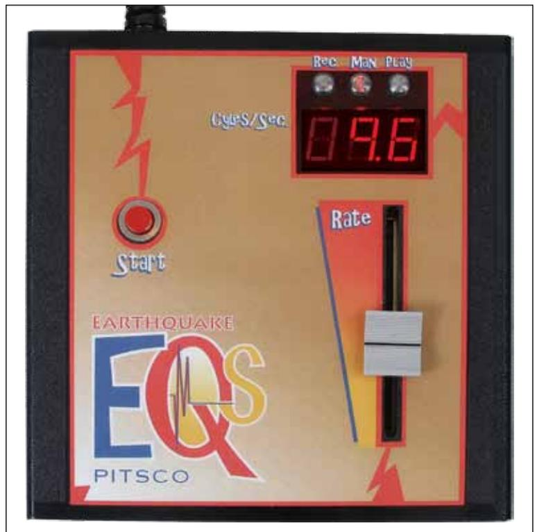
Figure 7 – Moving the Rate control slide changes the frequency.
