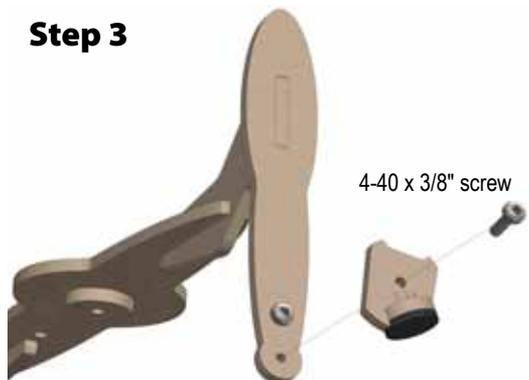
4. Now, loosely attach the B-15 feet with 4-40 x 3/8" screws to the Parts 4 and 6 subassembly (hips) so the toes point in the same direction.
