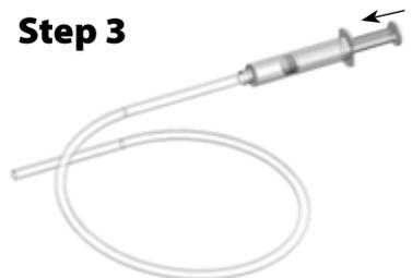
4. With someone holding the tube with the ends up, detach the syringe and refill it. Carefully lifting one tube end until the water comes as close to the other end without spilling, reattach the tube to this end and slowly depress until the tube is completely full of water.
