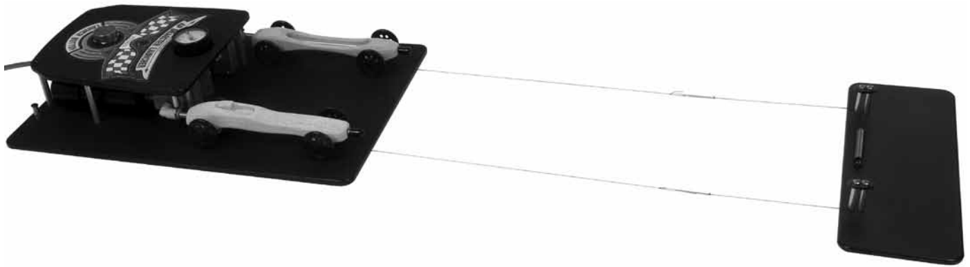
Figure 3 – the above image demonstrates the placement of the finish plate (at right) – it is not a proper length track
