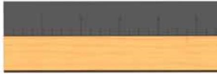
4. Glue the strip into the precut notches of the small base pieces so that the mark lines up with an outside edge of the base. The strip should be centered over the base.
