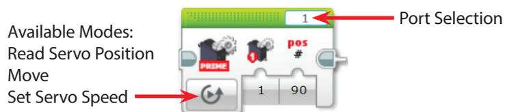
Note that the port in the top right must match the sensor port to which the module is attached for the block to function.
