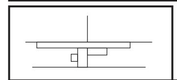
Make sure the wing saddle is at a right angle to the fuselage, and that it's level with the top. The wing should be flat and level with the stabilizer when viewed from the front. If it's still a little crooked after being rubber banded, use the sanding block to plane the saddle to the correct angle.
