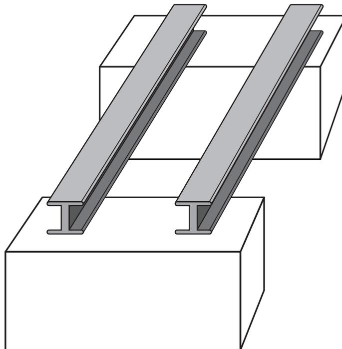
Position two I beams lengthwise across the span (above), then place the bridge deck on top of the beams.
