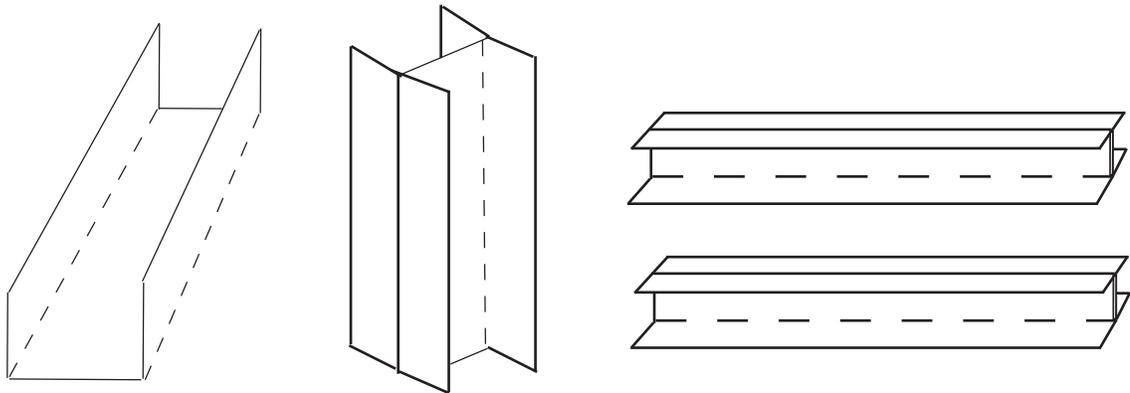
Make your own I beam! First, make two paperboard U channels (left), and then glue or tape them together back to back to make an I beam (middle). To support the bridge deck, you will need to make two I beams and position them vertically across the bridge supports as shown below.
